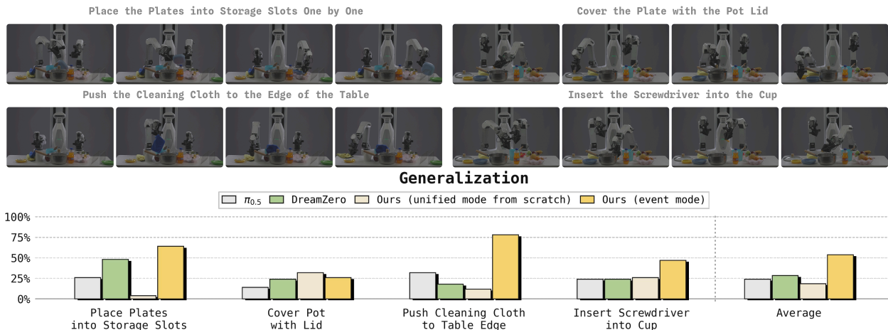
Figure 19 Real-robot Generalization benchmark. Task Progress scores in a complex tabletop scene where different instructions are issued in randomized order, testing scene grounding and compositional transfer.
