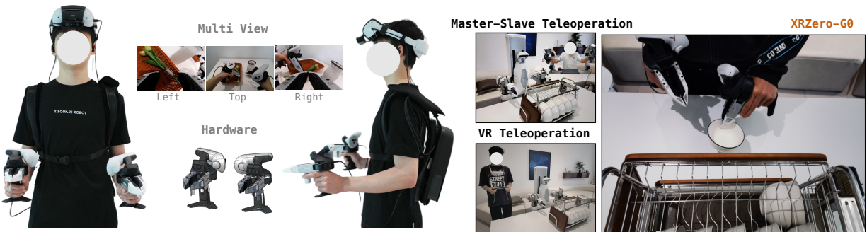
Figure 10 XRZero-G0 no-embodiment collection rig and its place alongside teleoperation (73). (Left) The wearable rig from two views: a VR-tracked headset carries three egocentric cameras (one top + two wrist-side feeds shown), an operator-borne backpack handles synchronization and edge-side compute, and a pair of handheld grippers reproduces the deployment robot’s end-effector geometry; the inset thumbnails show the three on-rig views (left wrist / top / right wrist) that the policy will eventually consume. (Right) XRZero-G0 sits alongside master-slave and VR teleoperation rather than replacing them: in the production recipe a small real-robot anchor fraction (the two teleoperation modes) is paired with a much larger no-embodiment volume (the XRZero-G0 rig), realizing the few-shot physical-anchoring regime characterized in (73).
